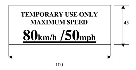
Upper case letters shall be at least 5 mm high and the numbers "80" and "50" shall be at least 20 mm high with the elements that make up each character of the number at least 3 mm line thickness. Lower case text shall be at least have a line height of 5 mm. All text shall be enclosed in a border and be on a background of contrasting colour.
