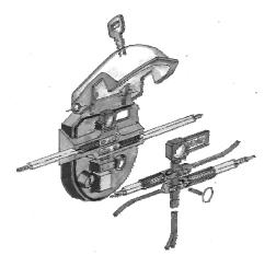
14. Positioning of the cable endings is ensured by a special housing installed at the back of the load compartment. Light impulses are let through the cable continuously. Should the cable be damaged or cut, the light impulse is not any more received by the optic sensor of the electronic unit, which immediately triggers the alarm at the surveillance center.
