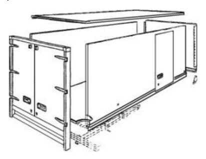
1.2 Parts of importance to the overall heat transfer, such as door-joints, must be of original brand and type. Parts of no importance to heat transfer, such as protection rails, hinges and meat bars, might be of a comparable brand.
