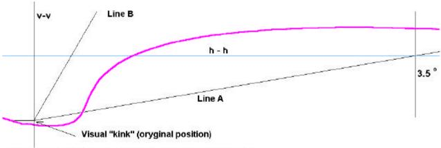
View of cut-off line before calculating of the aiming position of the "shoulder line part".
