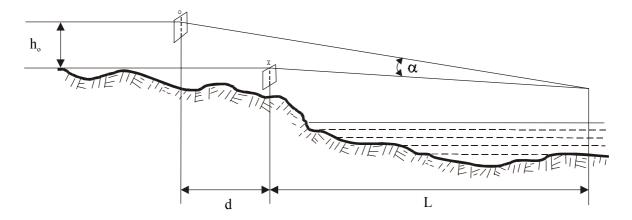
The value "a" in the table describes the precision of the alignment. The value is very important when the vessel passes through a narrow channel. As a rule, the precision increases the closer to the marker post.
