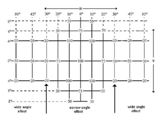
"Minimum horizontal angular range of category "narrow angle effect" is 30° left to 30° right and for category "wide angle effect" 90° directed outwards the vehicle and 30° to the inside.
