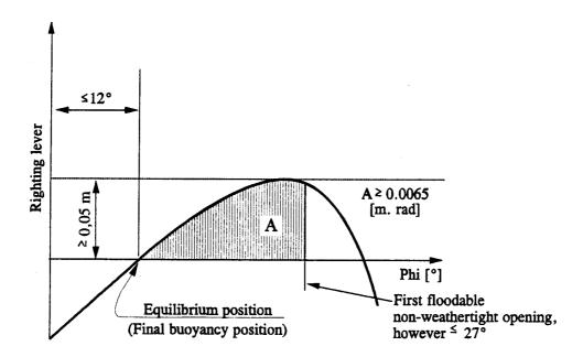
9.1.0.95.3 Inland navigation vessels carrying containers which have not been secured shall satisfy the following damage stability criteria.
