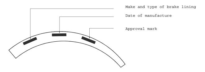
$\underline{\text{Note}} \colon \text{Positions}$  of markings and mutual positions of markings shown in the examples are not mandatory.
