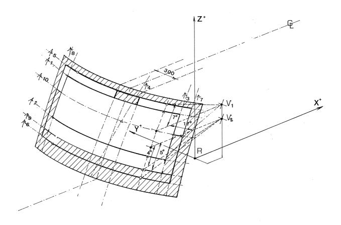
$C_{L}$ : trace of the longitudinal median plane of the vehicle  $P_{i}$ : trace of the relevant plane (see text)
