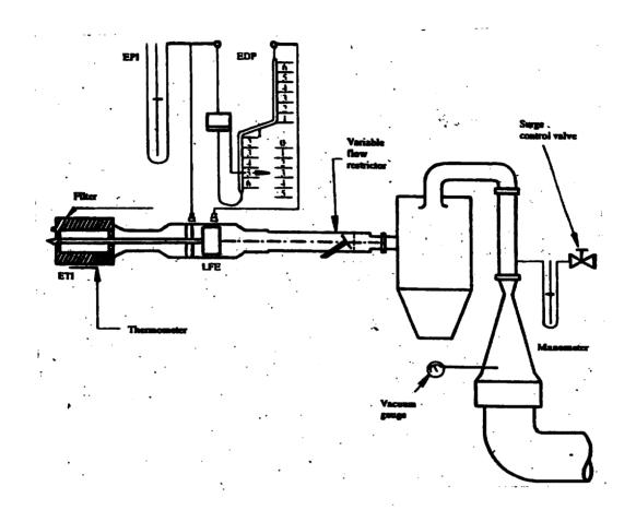
4.2.4.3. A CVS system that has multiple speeds shall be calibrated on each speed used. The calibration curves generated for the ranges shall be approximately parallel and the intercept values  $(D_{\scriptscriptstyle 0})$  shall increase as the pump flow range decreases.
