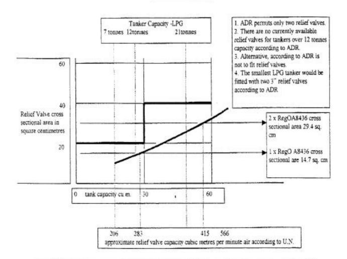
ADR requires 20 square centimetres of aggregate cross sectional area per 30 cubic metres or part thereof of tank capacity. The illustration shows that from the smallest capacity tanker to one of 30 cubic metres - 20 square centimetres of relief valve area is required. For a 31 cubic metre tank - 40 square centimetres of relief valve area is required. Only 2 relief valves are permitted.
