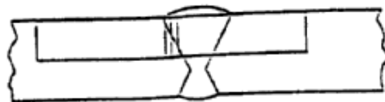
Heat affected zone
