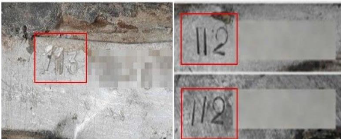
Figure 7: Numerical mark stamped on the jet vane actuator per CAR analysis
