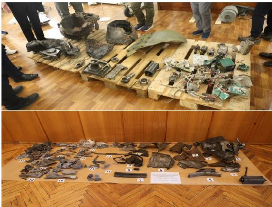
Figure 5: Remnants of Hwasong-11A short-range ballistic missile obtained in Ukraine
