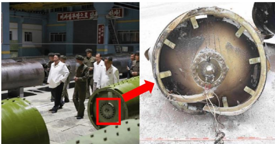
Figure 6: Front end of the rocket motor of a DPRK missile (left) and the rocket motor documented by CAR in Ukraine on January 11, 2024 (right)
