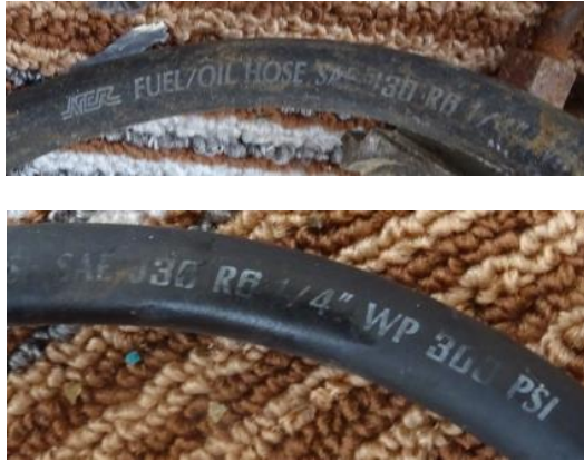
Figures 51.56. (up) and 51.57. (down) NCR fuel/oil hose
