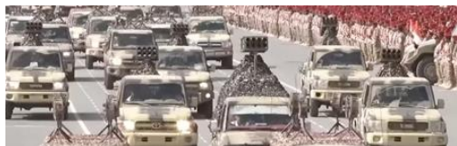
Figure 65.17. Mounted with 122mm MLRS with six tubes
