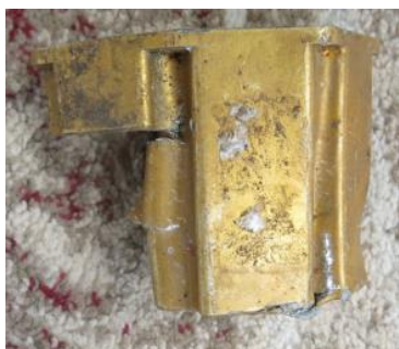
Figures 51.19. (up), 51.20. (centre) and 51.21. (down) Part of one of the three actuator systems (housing of servo motor) with serial number starting with "211"
