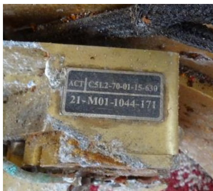
Figure 51.24. Marking of one of the three actuator systems
