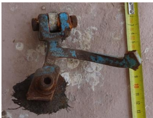
Figure 51.48. Broken jet engine suspension bracket
