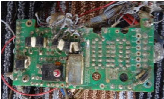
Figure 51.40. Electronic circuit board (ECB) of battery box
