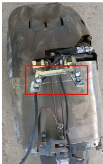
Figure 51.49. Jet engine suspension bracket of a cruise missile used in the Houthi attack in September 2019 on ARAMCO installations in the KSA
