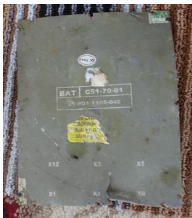
Figures 51.32. (up) and 51.33. (down) Battery box front plate
