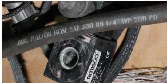
Figure 51.58. NCR fuel/oil hose of a cruise missile used in the Houthi attack in September 2019 on ARAMCO installations in the KSA
