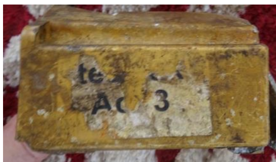
Figure 51.28. Part of the actuator systems #3 (housing of servo motor) with “test ok / Act 3” sticker
