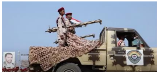
Figure 65.7. Mounted with 82mm recoilless gun similar to B10 or a variant of it
