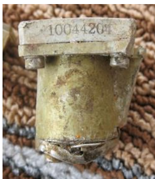
Figure 51.60. Jet engine component with serial number in the format "100XXXXX" (100 followed by five digits)
