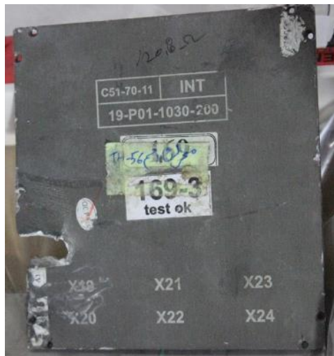
Figures 51.47. Interface box front plate found among the debris of a cruise missile used in a Houthi attack on Abu Dhabi airport, UAE, in January 2022
