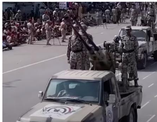
Figure 65.6. Mounted with 37mm twin-barrel anti-aircraft canon Type 65 or a variant of it
