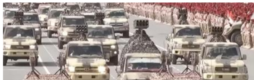
Figure 65.17. Mounted with 122mm MLRS with six tubes
