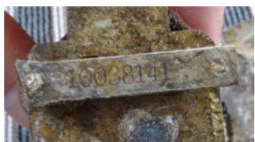
Figure 51.59. Jet engine component with serial number in the format "100XXXXX" (100 followed by five digits)
