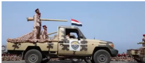
Figure 65.10. Mounted with 106mm recoilless gun similar to M40 or a variant of it
