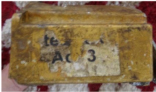
Figure 51.28. Part of the actuator systems #3 (housing of servo motor) with “test ok / Act 3” sticker
