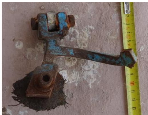
Figure 51.48. Broken jet engine suspension bracket
