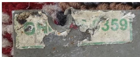
Figure 51.76. Close-up of battery box part “GH... 0359” sticker
