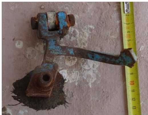
Figure 51.48. Broken jet engine suspension bracket
