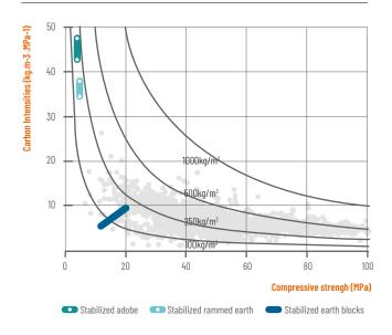
Stabilisation of earth masonry using Portland cement multiplies the carbon intensity index.
