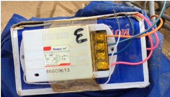
Figure 3: Learning code receiver model Honest number 66609613 found in captured IED
