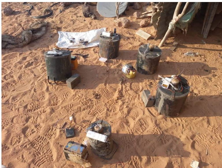
Figure 9: Five IEDs with explosives in sections of 13 inch steel tube with batteries, MC, LCR and remote controls
