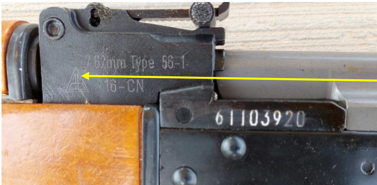
Figure 3: Marking: 7.62mm Type 56-1; logo (26 inside a triangle); 16 – CN; Serial 61103920
