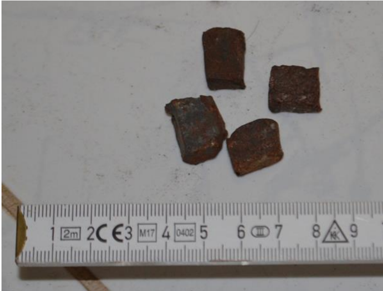
Figure 7.15 Metal cubes which were part of the fragmentation warhead of the missile
