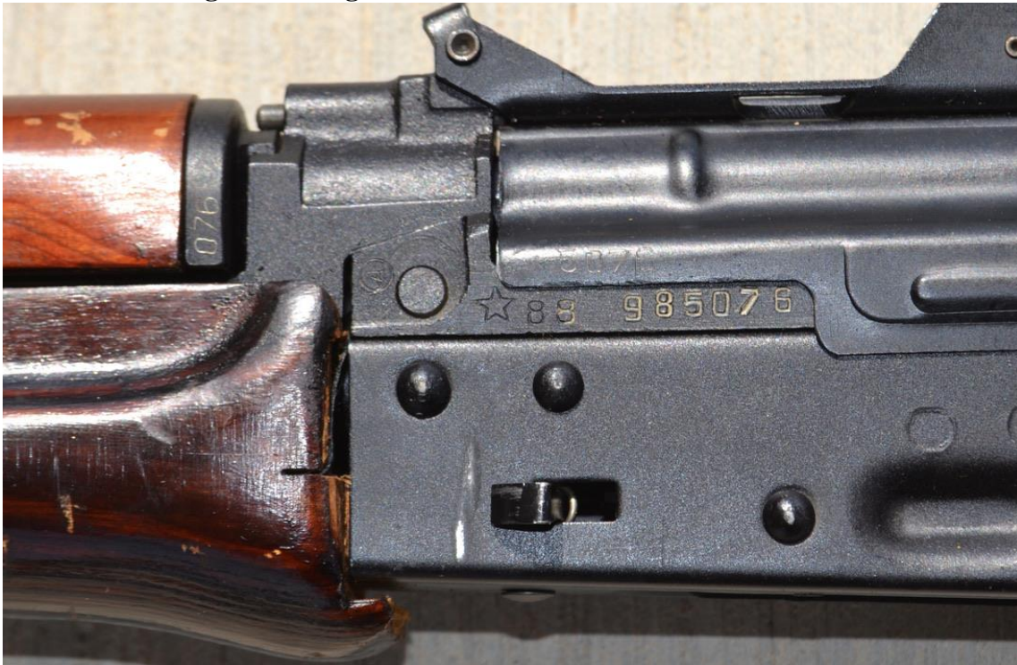
Figure 20.29 Detail of markings indicating manufacture at the Tula Arms Plant in 1988
