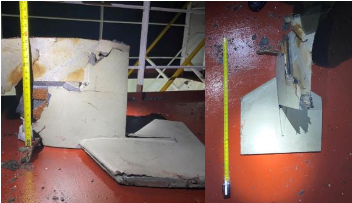
Figure 15.5 Vertical stabilizer of the UAV
