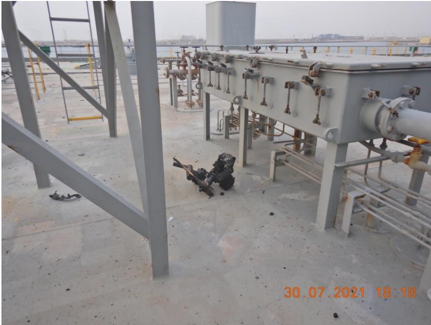
Figure 14.4 Debris of the engine of the UAV
