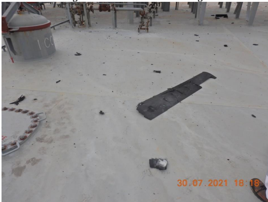
Debris of the wing of the UAV made from fiberglass
