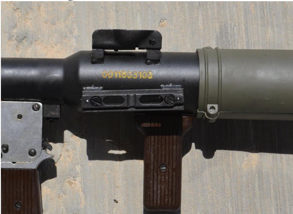
Figure 20.18 Detail of marking on RPG-7 launchers
