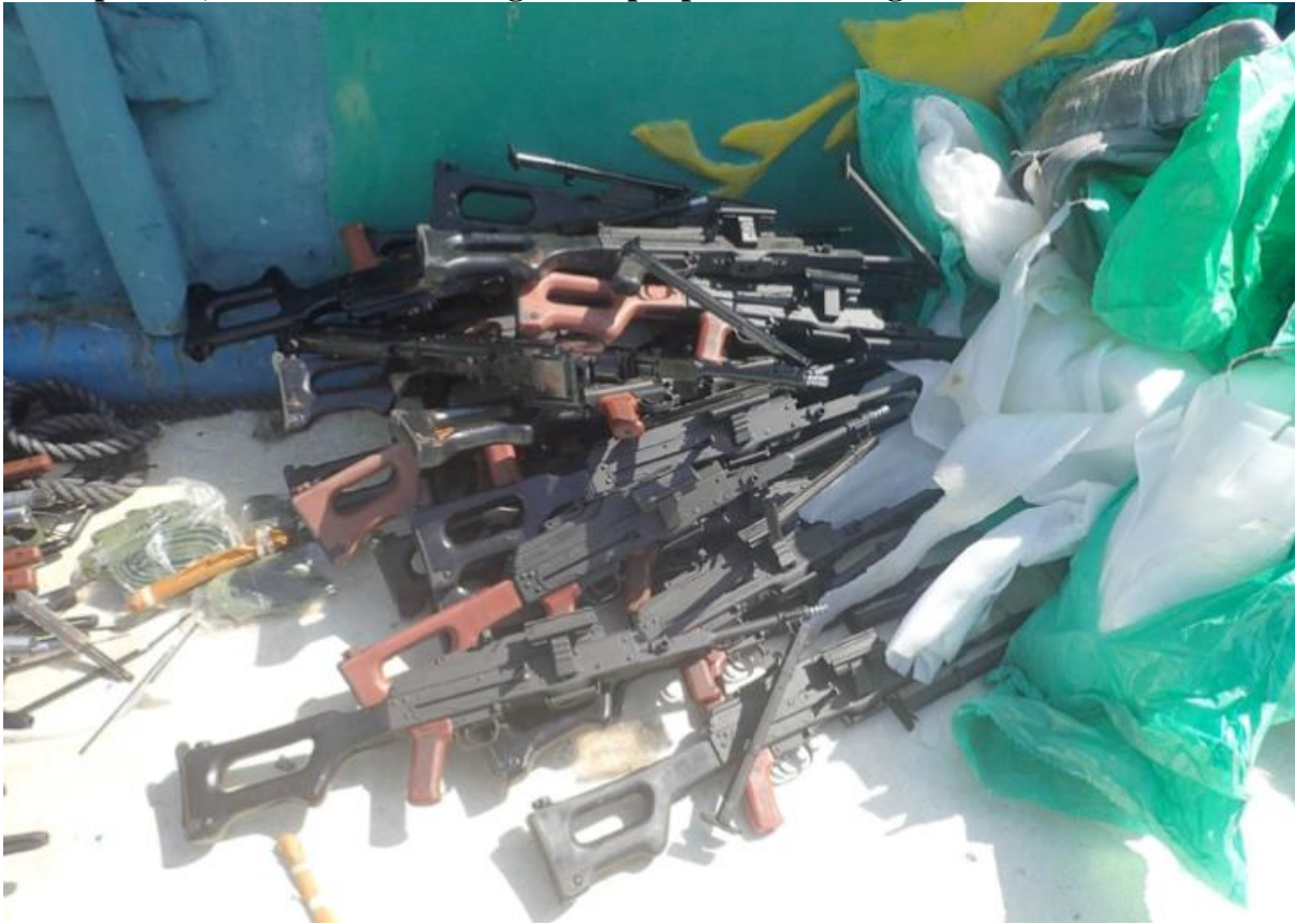
Figure 19.7 PKM-pattern, 7.62x54mm calibre general-purpose machine guns
