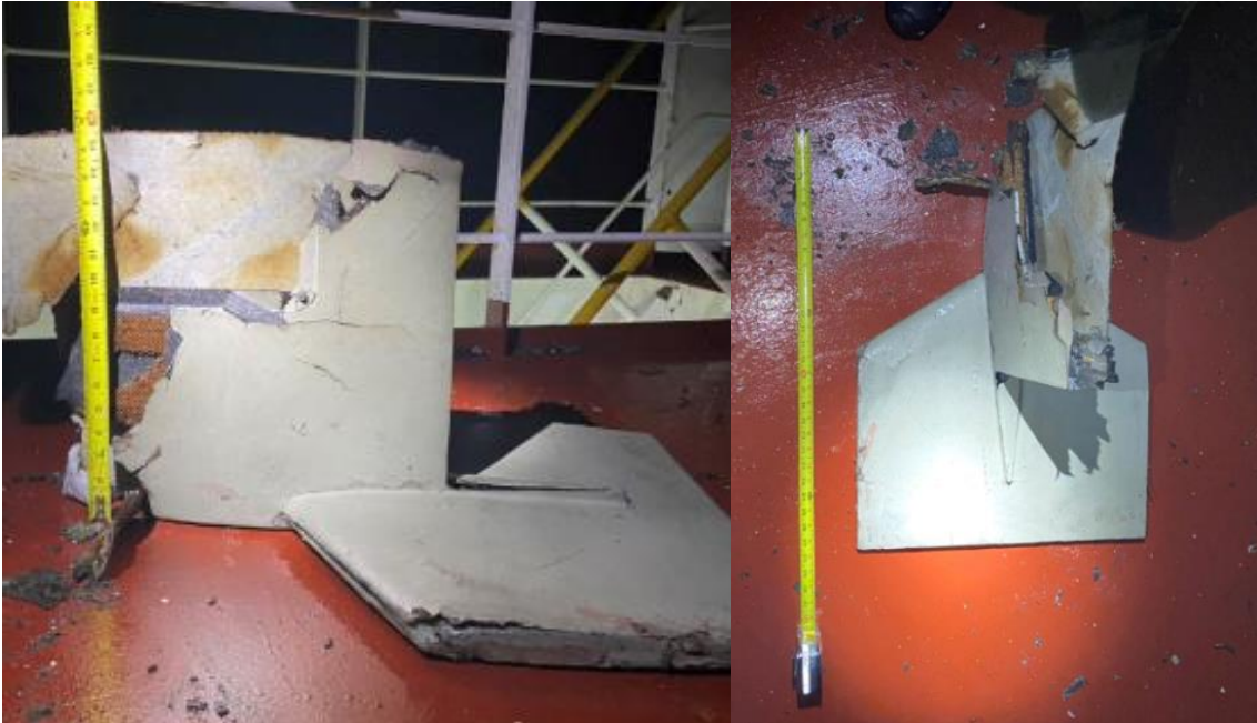
Figure 15.5 Vertical stabilizer of the UAV
