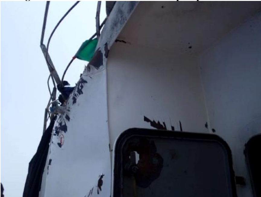
Figure 15.4 Damage to exterior bulkhead below the impact point
