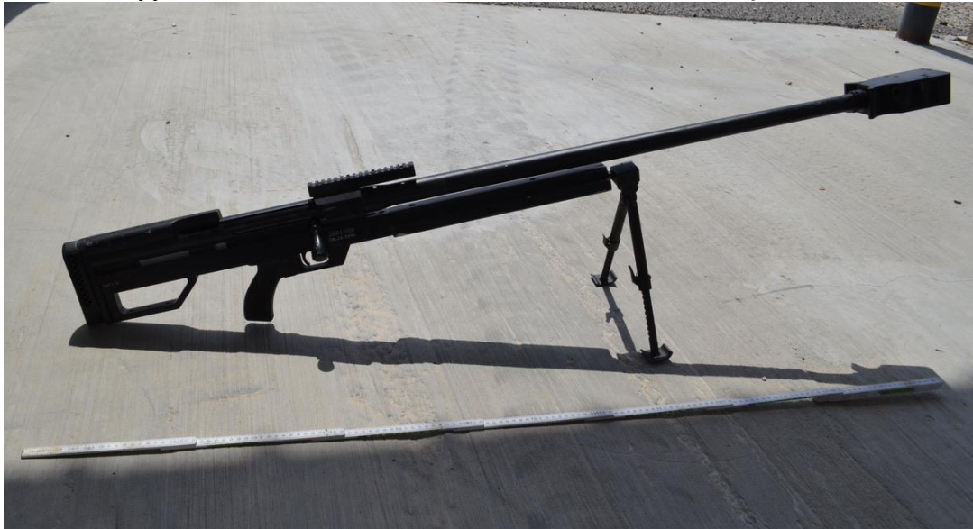
Figure 20.19 AM-50 ‘Sayyad’, 12.7x99mm calibre anti-material rifle, likely manufactured in Iran 238
