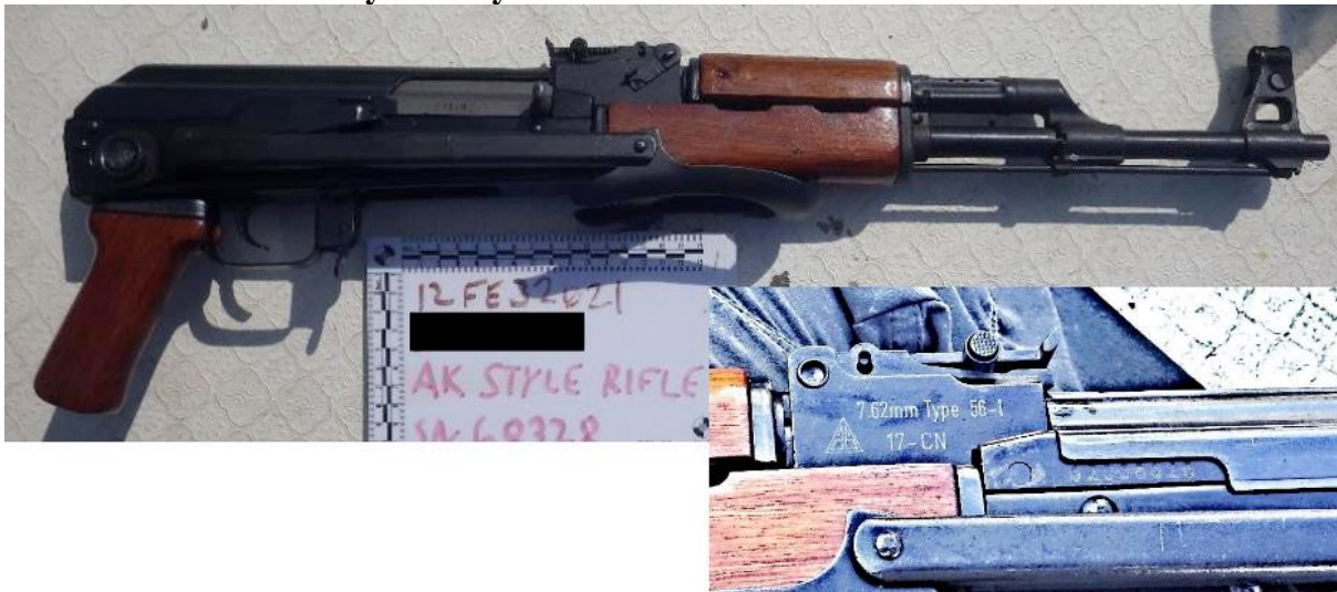
Figure 19.6 Type 56-1, 7.62x39mm assault rifle and detail of the markings showing that the weapon was manufactured in 2017 by Factory 26 in China
