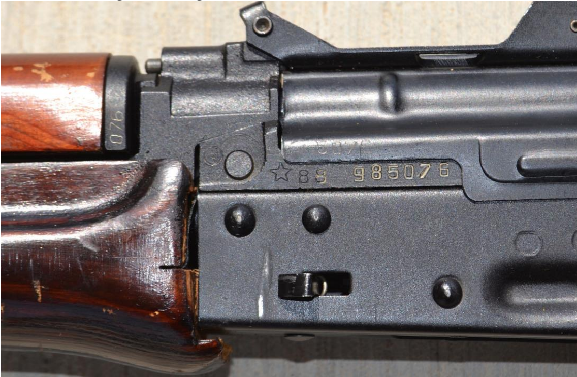
Figure 20.29 Detail of markings indicating manufacture at the Tula Arms Plant in 1988
