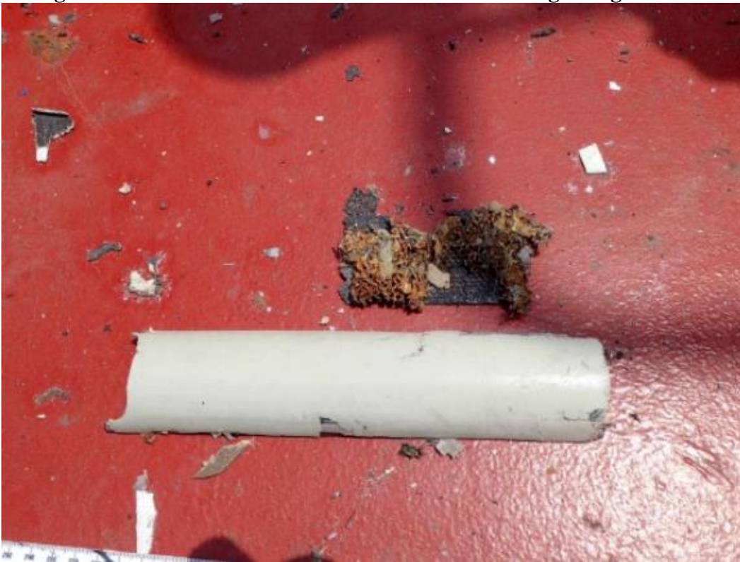
Figure 15.7 Fiberglass debris from the UAV recovered from the bridge wing
