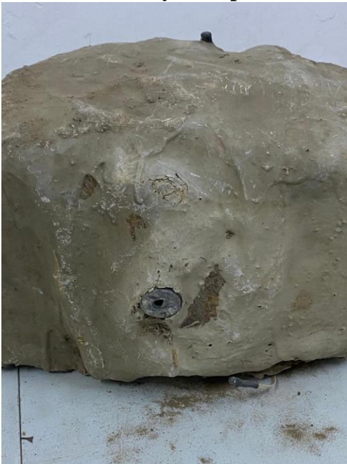
Figure 36.4: IEDs activation system: passive infra-red sensor
