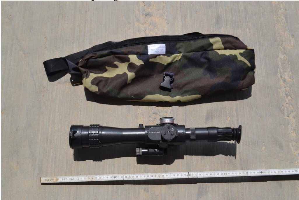
Figure 20.36 POSP 12x50M Telescopic Sight manufactured in Belarus
