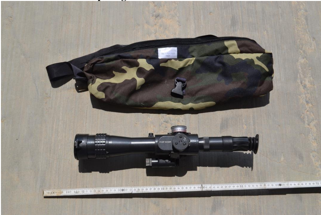
Figure 20.36 POSP 12x50M Telescopic Sight manufactured in Belarus
