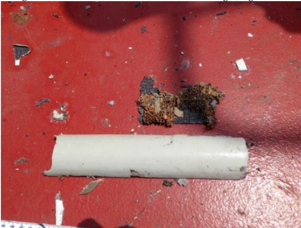
Figure 15.7 Fiberglass debris from the UAV recovered from the bridge wing
