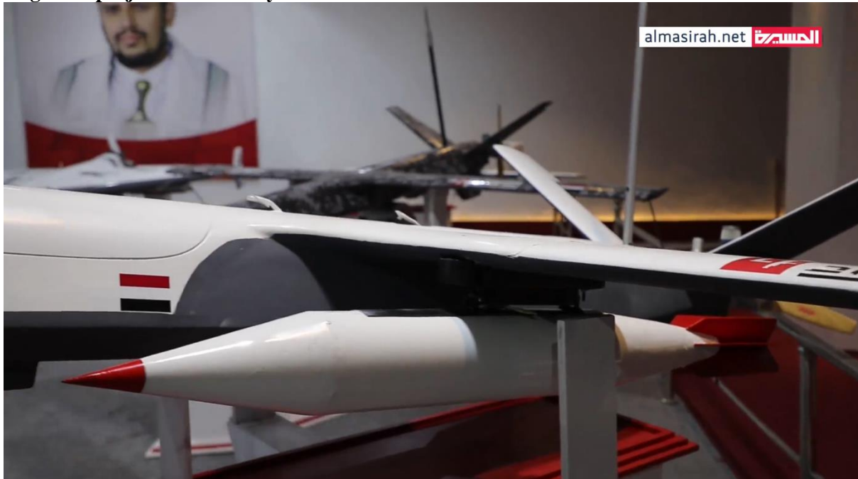
Figure 18.3 Unguided projectile carried by the SAMMAD-4 UAV
