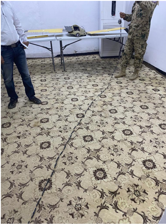
Figure 36.3: IEDs activation system: crush wire
