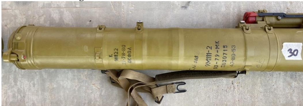
Figure 20.34 9M111-2 Anti-tank guided missile manufactured in Russia
