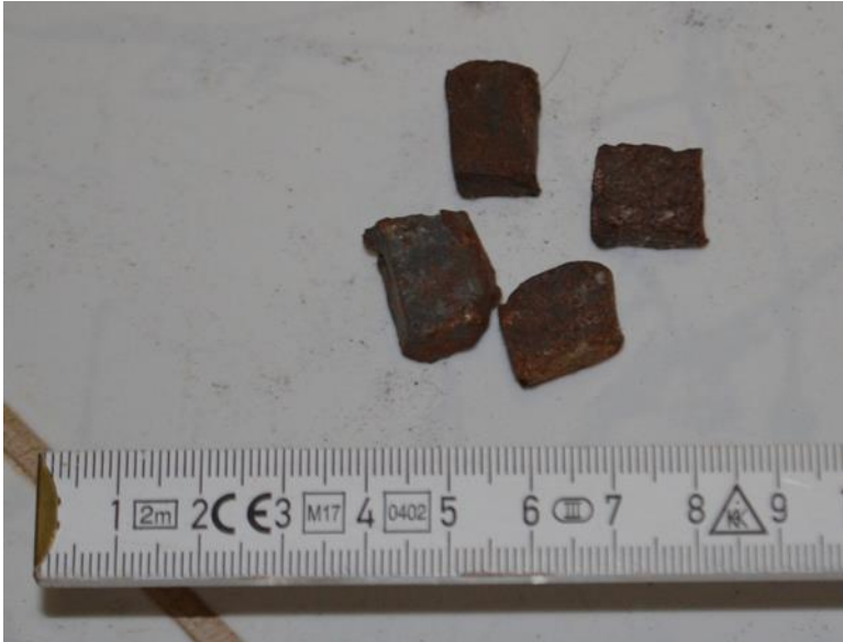
Figure 7.15 Metal cubes which were part of the fragmentation warhead of the missile
