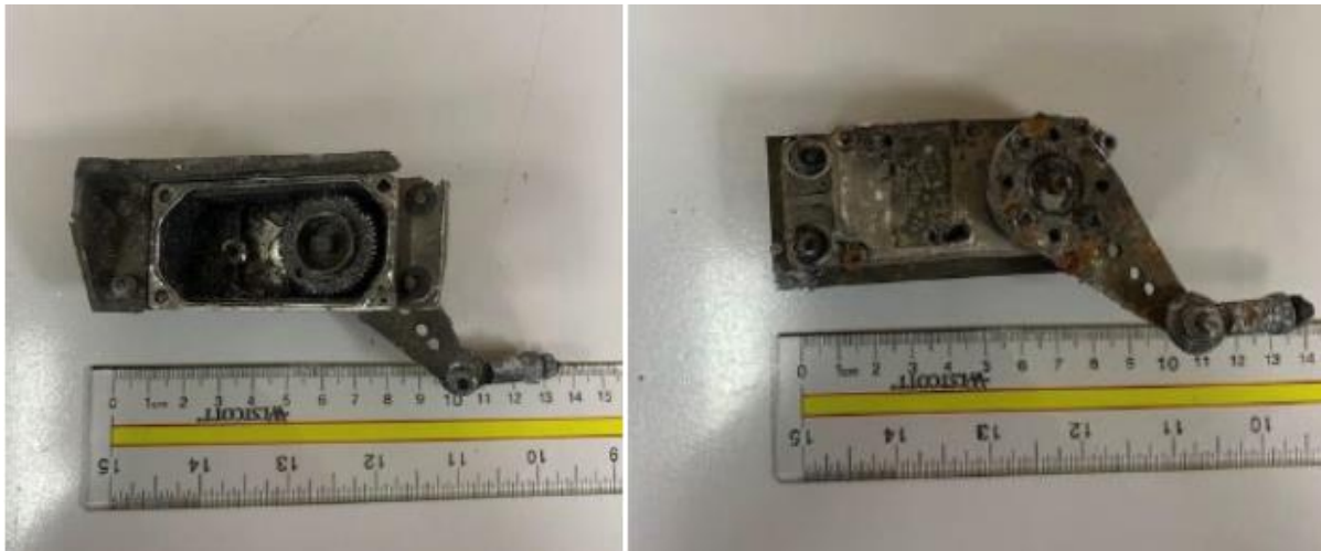
Figure 15.6 Debris of a servo actuator from the UAV
