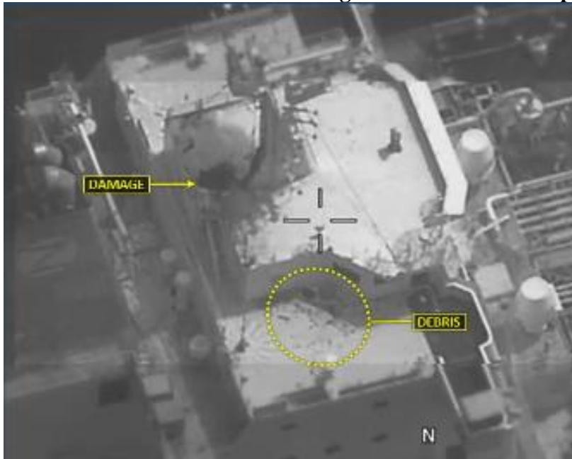
Figure 15.1 Aerial view of the aft castle showing the location of the impact
