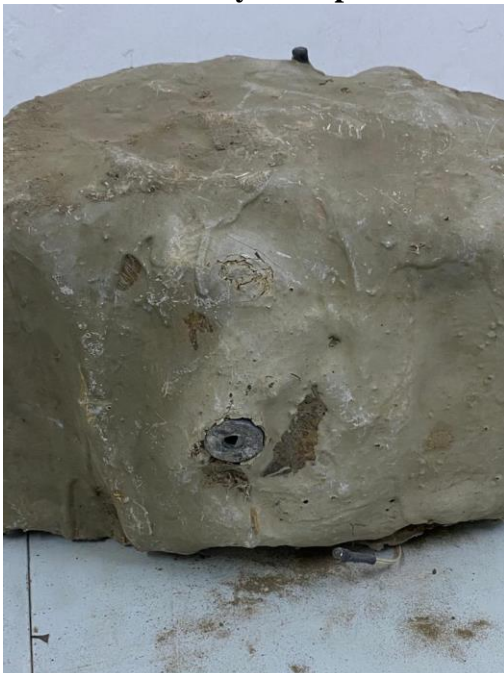
Figure 36.4: IEDs activation system: passive infra-red sensor
