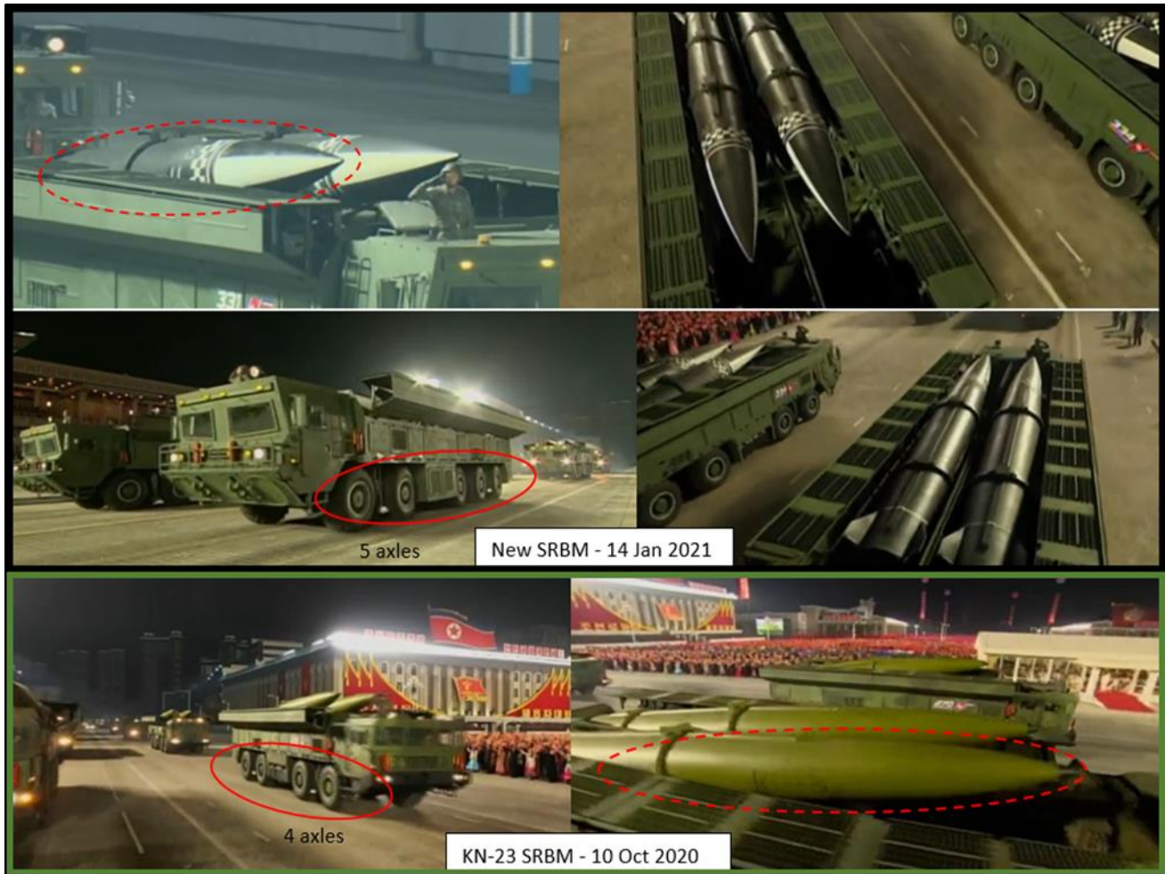
Figure 12-2: A new SRBM (resembles KN-23) was revealed in the military parade of 14 January 2021 in Pyongyang, broadcast by KCTV (new SRBM seems to be larger than KN-23 and its TEL has 5 axles)
