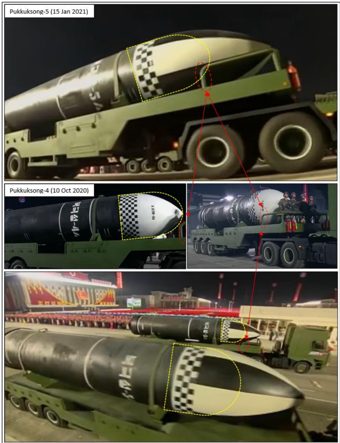
Figure 11-2: New MRBM/SLBM Pukguksong-5, larger than Pukguksong-4, was revealed in the military parade of the 14 January 2021 in Pyongyang (yellow dotted line marks the shroud of Pukguksong-4)
