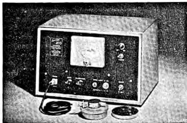
Figure 21. Front view of radioactivity comparator showing probe in position for testing unknown sample
