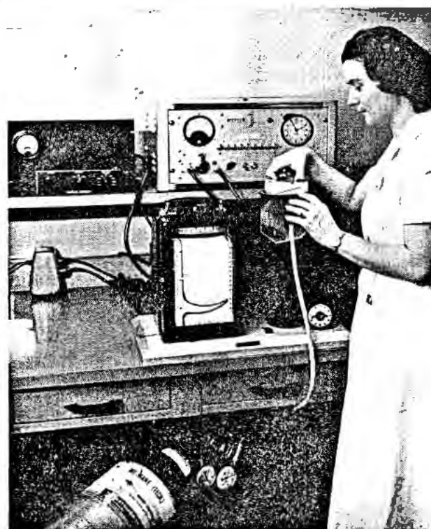
Figure 3. Methane gas flow counter for scanning paper chromatograms
