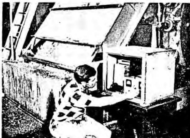
Figure 15. Bagasse stream falling between Cs^{137} source and receiver with recorder at right
