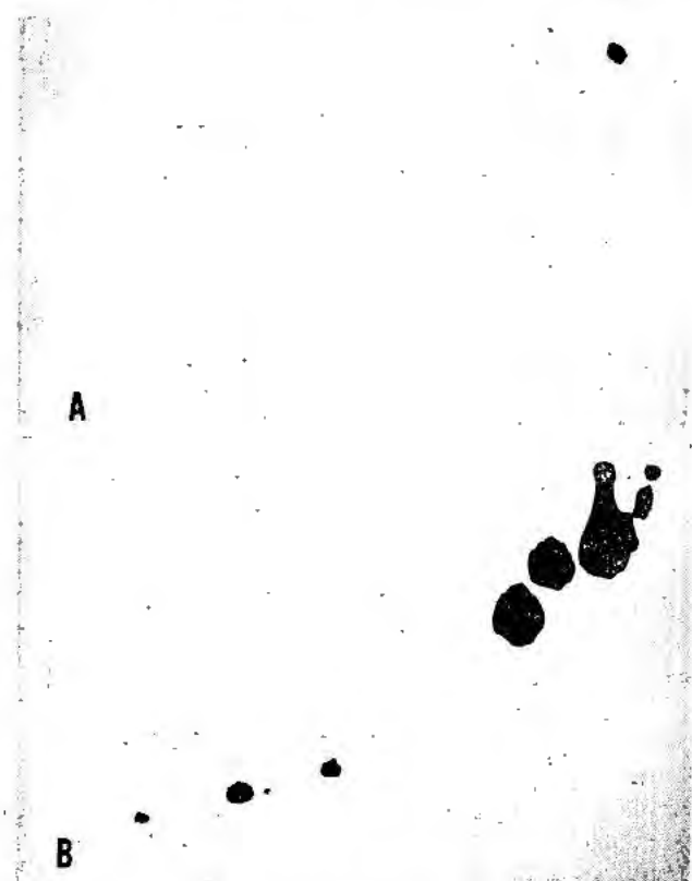
Figure 3. Chromatogram of compounds separated by paper chromatographic technique. (A), compounds detectable after chemical treatment; (B), compounds detectable when a radioautograph is made of the same chromatogram shown in (A)
