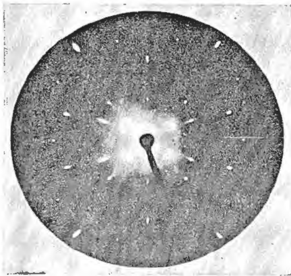
Figure 7. Diamond (110) laue transmission photograph
