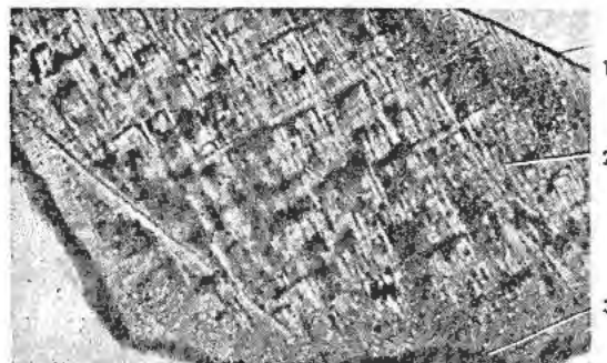
Figure 1. Uranium sheet after irradiation: (1) surface adjacent to steel; (2) sheet; (3) surface adjacent to magnesium
