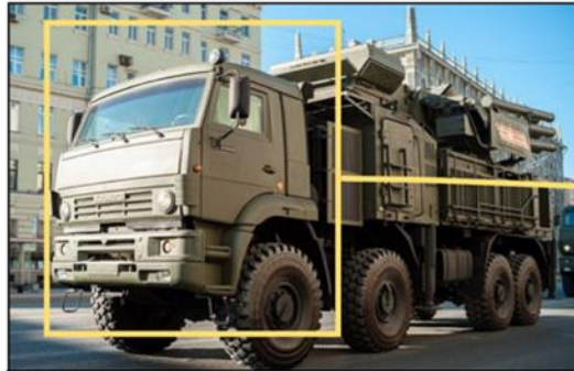
Production Pantsir S-1 on KaMAZ 6560 ground mobility platform. NOTE: Distinct driver cab differences: 1) sloping cab; 2) drivers steps; 3) front bumper; 4) window shapes; etc..
