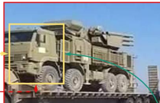
Pantsir S-1 on KaMAZ 6560 ground mobility platform in Libya on 12 July 2020. NOTE: Distinct driver cab difference to Pantsir S-1 previously identified as being in Libya 2019.
