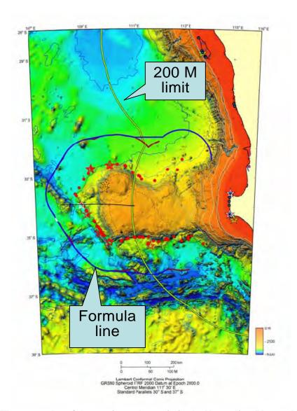
Figure F.3 The outer edge of the continental margin in the Naturaliste Plateau Region defined by the formula line established in accordance with article 76, paragraphs 4(a)(ii) and 7, as based on the foot of the continental slope points submitted by Australia on 15 November 2004 and revised as per AUS-CLCS-DOC-44 submitted on 1 September 2006.
