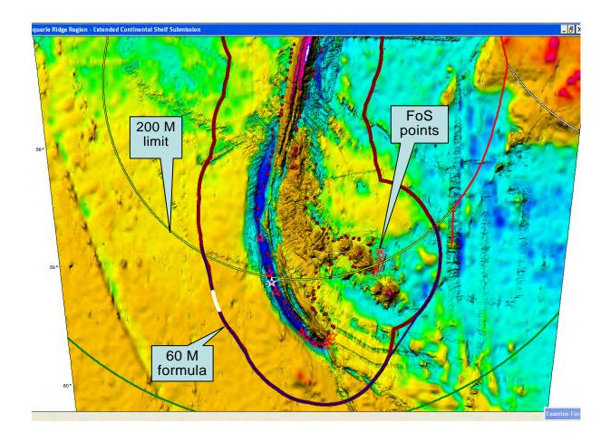
Figure E.2 Relationships between the 200 M limit, the foot of the continental slope points and the formula lines according the article 76. 4(a) in the Macquarie Ridge Region. White arrows point out saddle regions critical for the morphological continuity.
