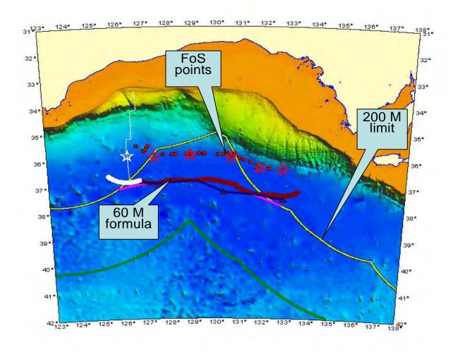
Figure B.2 Relationships between the 200 M limit, the foot of the continental slope points and the formula lines according the article 76. 4(a) in the Great Australian Bight Region.
