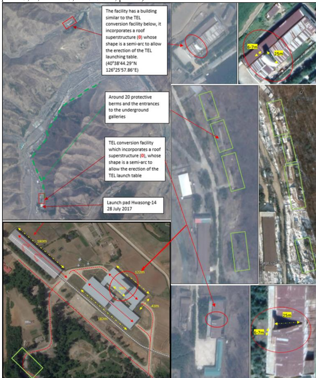
Figure 12-9: Comparison between structure of the possible ballistic missile support facility (aka Sil-li ballistic missile support facility) (39°10'50.56"N 125°39'50.01"E) and at the Jonchon-Mupyong-ni No 65 factory , the southern building involved in the TEL upgrading (40°36'42.77"N 126°25'34.74"E) and the various underground galleries located along the westside of the mountain from south (40°36'48.06"N 126°25'35.59"E) to north-east (40°38'0.43"N 126°26'21.20"E). A Hwasong-14 was tested on 28 July 2017 from a near-by launch pad (40°36'40.21"N 126°25'33.31"E) (see S/2019/171, para. 174; S/2018/171, paras. 9,11,12 and 13; S/2017/742, para. 7)
