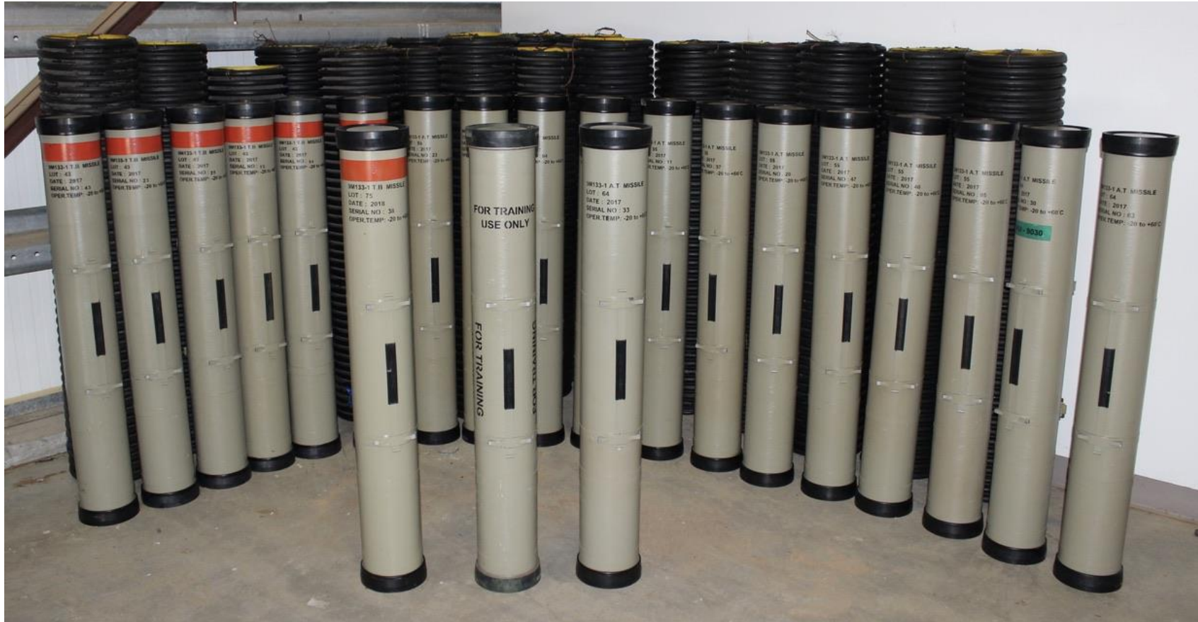
The launch tubes with the red band contain the thermobaric version of the missile, in the back are the transport containers. Source: Panel.
