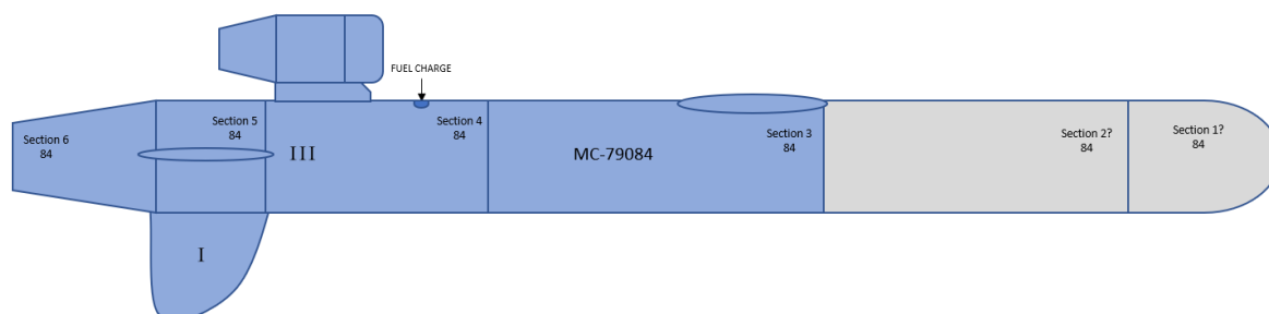
Figure 14.7 Schematic drawing of the Quds-1 cruise missile
