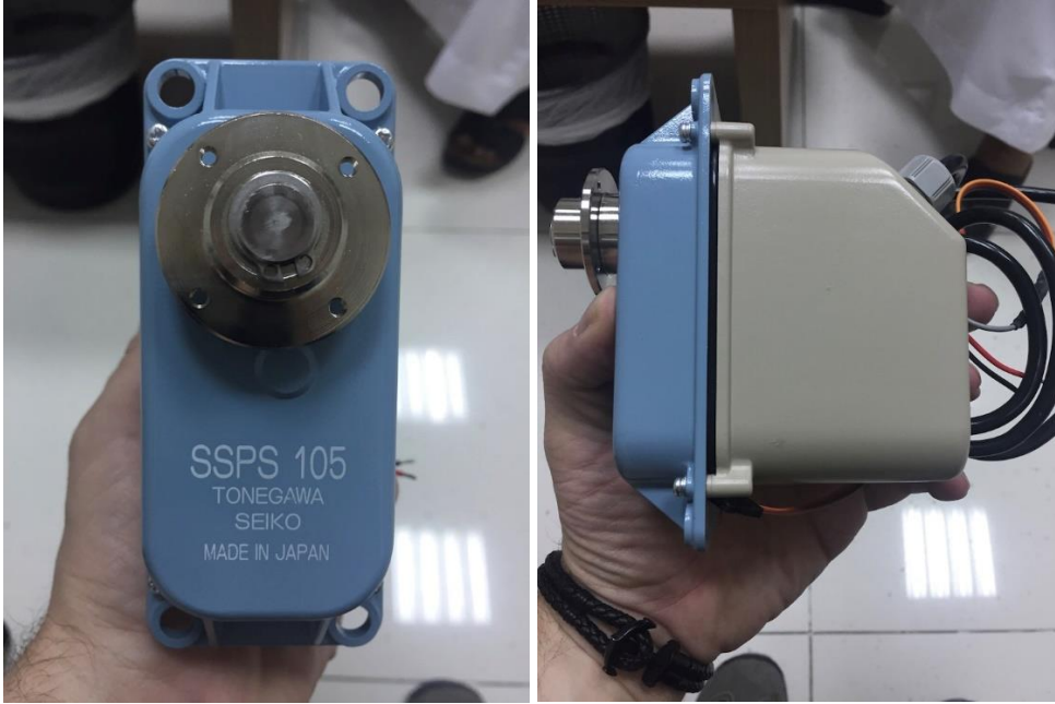
Figure 17.10 SSPS 105 Servo actuators seized in the UAE
