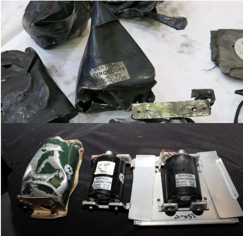
Figure 15.4 Vertical gyroscope inspected by the Panel (top), gyroscopes at the IMD (bottom)
