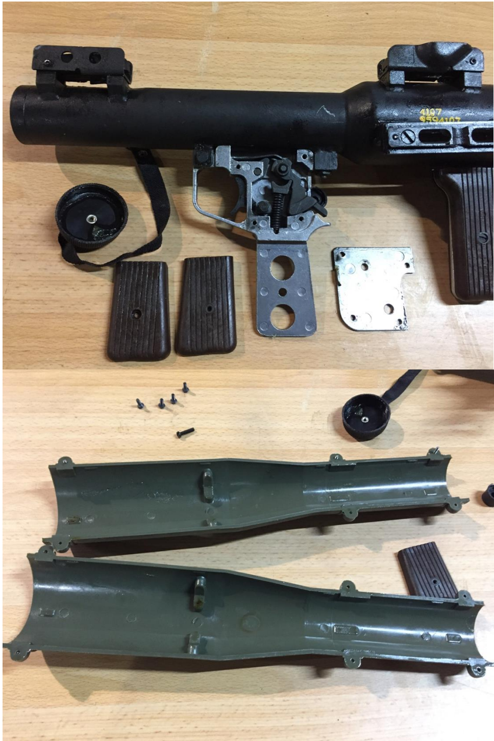
Figure 19.4 RPG-7 launcher seized by the Coalition in Aden, disassembled by the Panel
