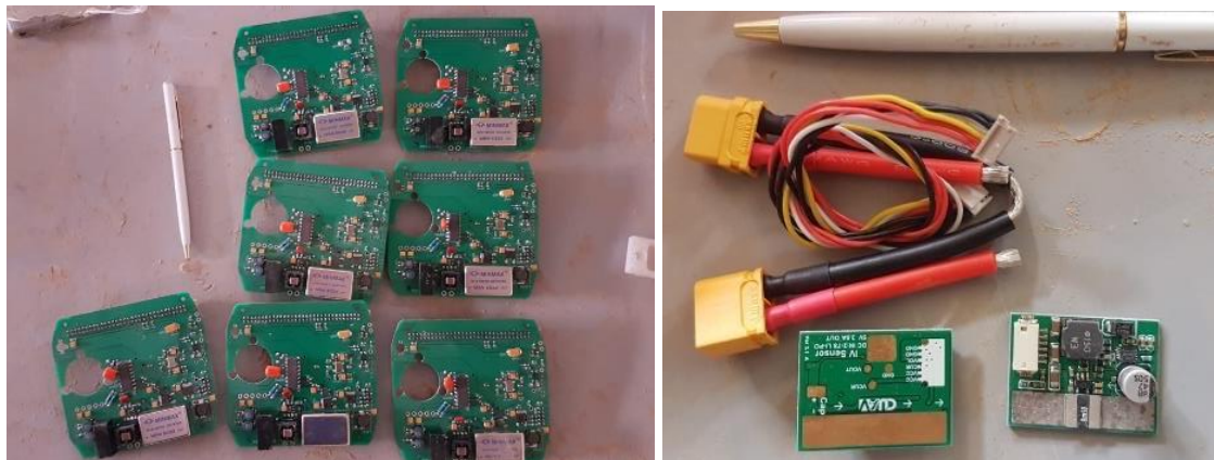
Figure 17.7 Components used in UAV guidance units in Al Jawf
