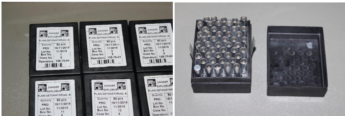
Figure 20.12 Non-electric detonators – a total of 13,700 in boxes of 50 each
