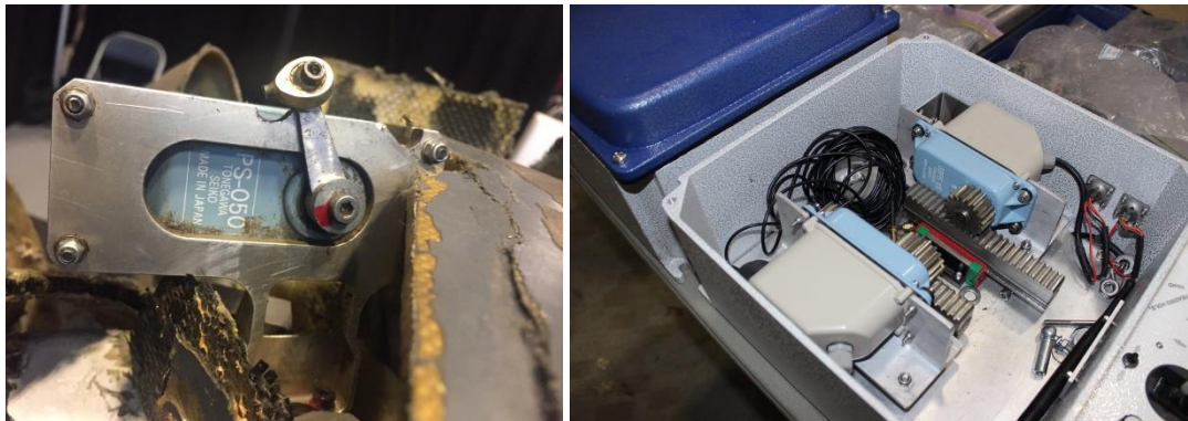
Figure 17.11 SSPS servo actuators in a 'Shahed-123' UAV (left) and in the steering box of a WBIED (right)
