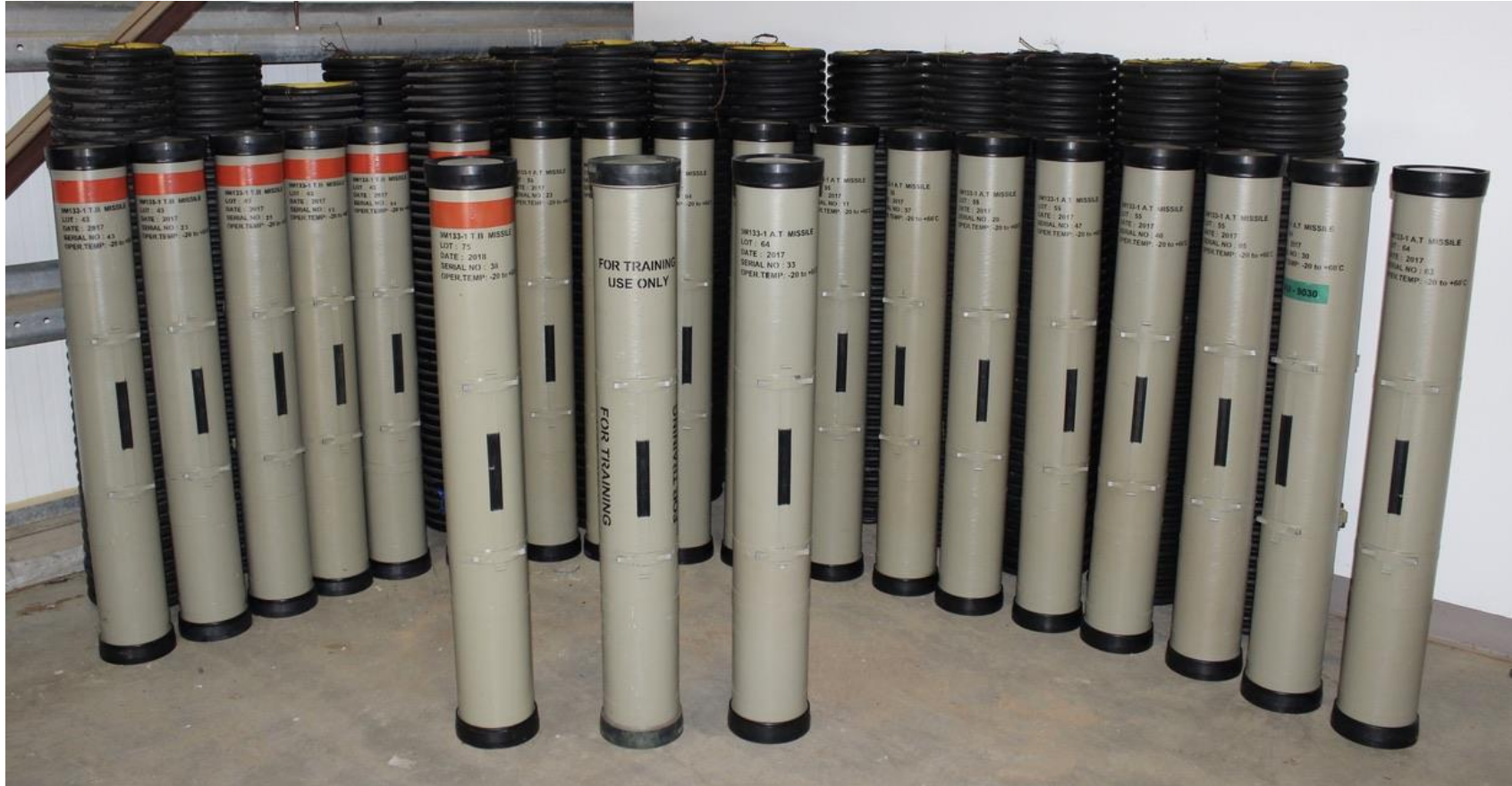
The launch tubes with the red band contain the thermobaric version of the missile, in the back are the transport containers.
