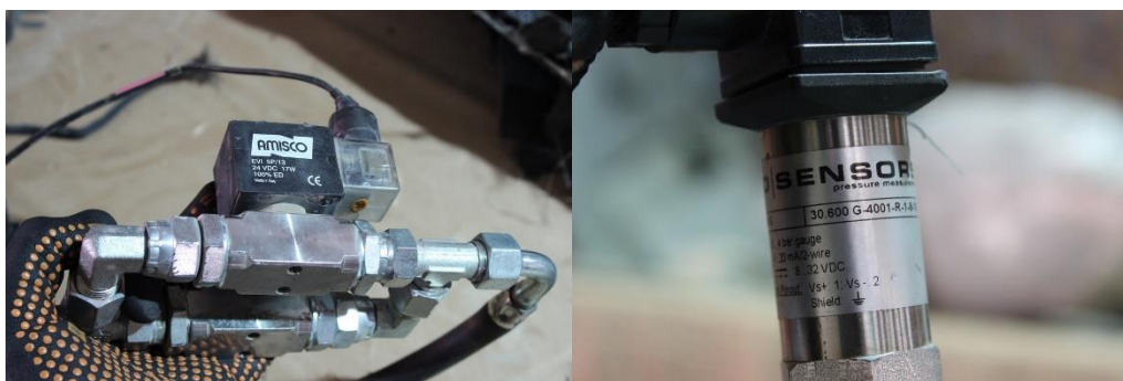
Figure 16.4 Commercial components documented as part of the LACM's fuel system
