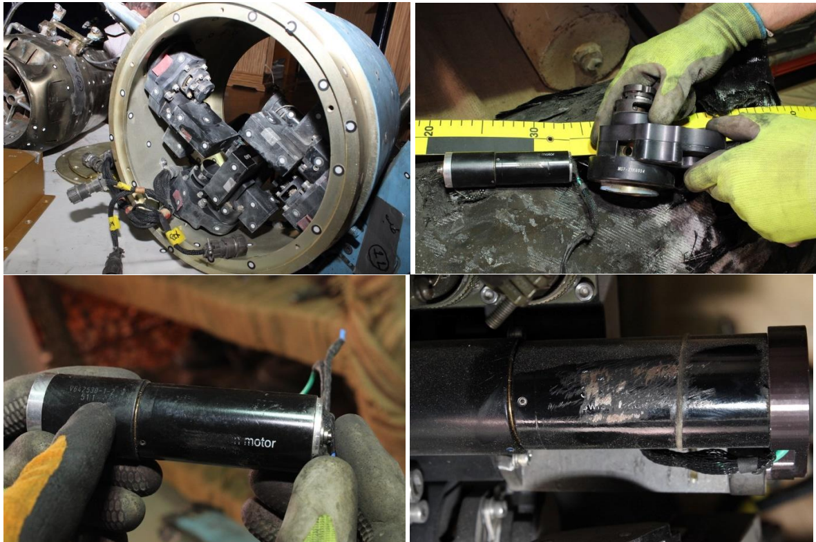
Figure 16.3 Servo actuators documented among the debris of the LACM
