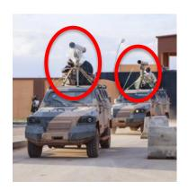
Figure B.36.3 KADDB Al Wahsh PPV modified with an 73mm SPG-9 recoilless gun fitted to 'snakehead' cupola c
