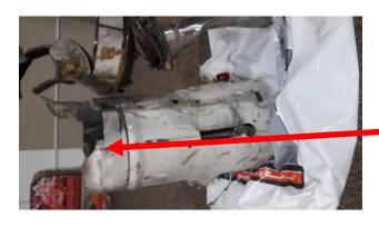
A. Imagery of missile remnant Note: Reduction in fuselage diameter (identifiable after "trumpeting" due to impact)
