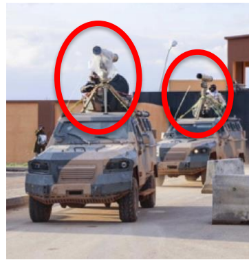
Figure B.36.2 Streit Cougar LAMV modified with a 9M133 Kornet ATGW b
