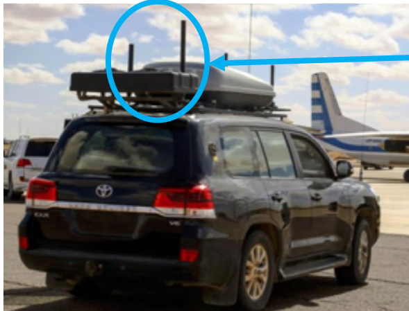
Image 41.1 HAF ECM equipment at Tamanhint (Sebha) air base (13 February 2019)
