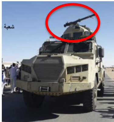
Figure B.36.3 KADDB Al Wahsh PPV modified with an 73mm SPG-9 recoilless gun fitted to 'snakehead' cupola c
