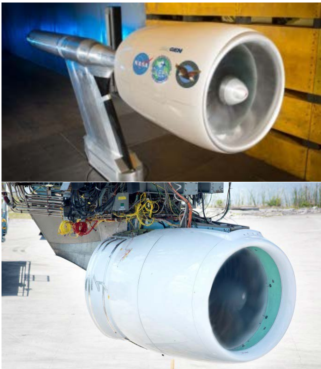
FIGURE 4: NASA ERA Wind-Tunnel Test (Top), FAA CLEEN Phase-I High BPR, Short Inlet Fan Rig and Engine Demonstrator Program (Bottom)
