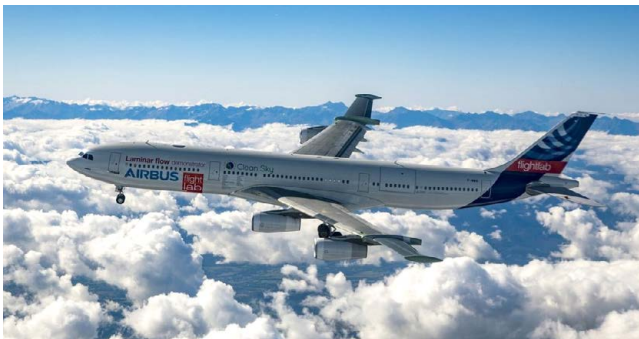
FIGURE 2: Integrated wing NLF (Natural Laminar Flow) integration concepts installed on modified outboard wings of A340-300 (Clean-Sky 2 flight demonstrator BLADE) (Ref. 3)
