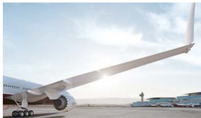
FIGURE 1: On-ground folding wing tip to maximize in-flight wing span (Boeing B777-9) (Image courtesy Boeing)
