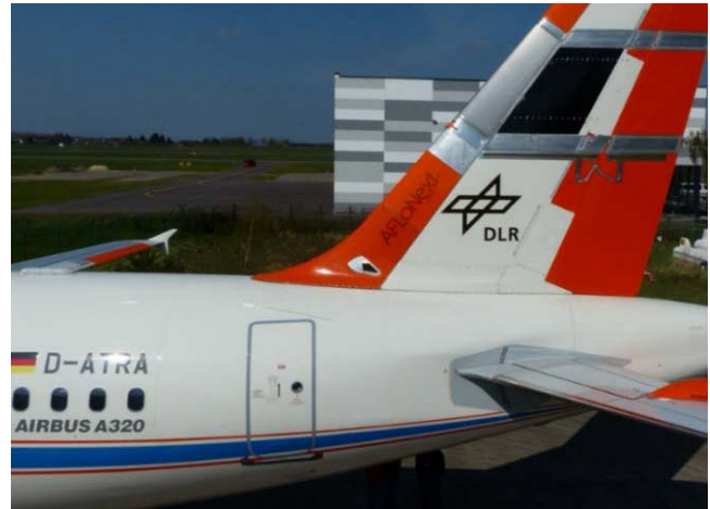
FIGURE 3: AFLoNext HLFC empennage flight test on DLR's A320 test aircraft (Image courtesy DLR)
