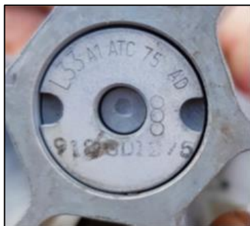
Figure 1: Base stamp from a primary propelling cartridge of one of the recovered fin assemblies from the 1 July 2018 attack on the airport's Jazeera gate.
