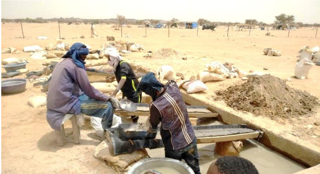
Washing process (with soap) of crushed stones in a site located four kilometres north of Kidal, at 31QCA2984643035
