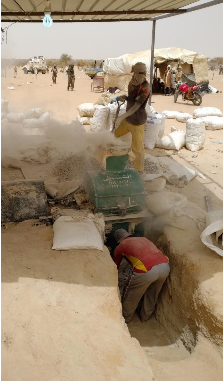
Crushing of stones extracted from a gold mining site before washing process in a site located four kilometres north of Kidal, at 31QCA2984643035
