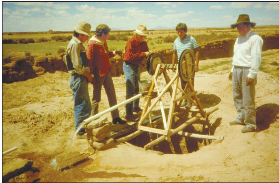
Ambrosio’s home-made FLOM well and pump. If he can make it, he can fix it; thus it is more reliable than if he were dependent on outside technicians.
