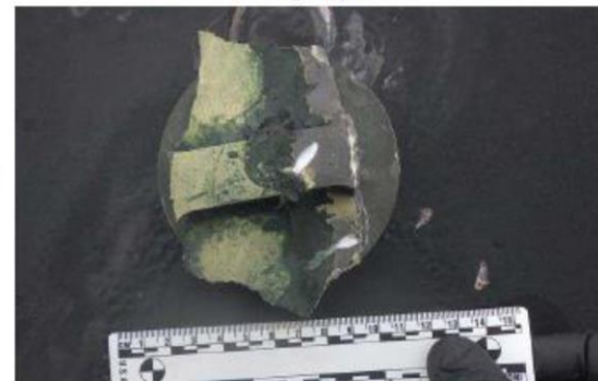
(U) Magnet 3.5" diameter; aluminum, composite remnants
