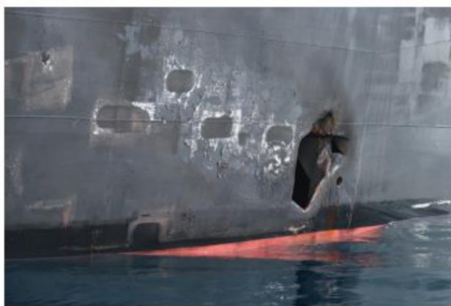
7725 - This photo is a view of hull penetration/blast damage sustained from a limpet mine attack on the starboard side of motor vessel M/T Kokuka Courageous, while operating in the Gulf of Oman, June 13.
